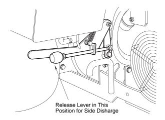
Figure 4-10 Side Discharge Operation Position
